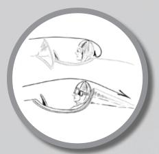
How airflow and drag are affected by cockpit design (credit: Scott Cullen)
