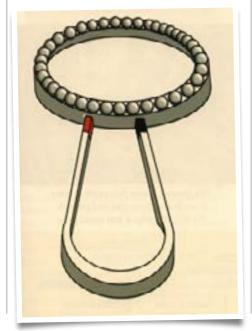
I love the simplicity of this next item from 'Roadholder' the magazine of the **Norton Owners Club**. Headed 'A load of balls', I will give it to you in full. "A neat idea from the past - many are aware of the trick of applying lashings of grease on the ball tracks of head bearings etc., when assembling forks/ yokes- it works but can be messy. An alternative solution is to use a magnet held against the steering head – this in turn temporarily magnetises the head and holds the balls in place."
