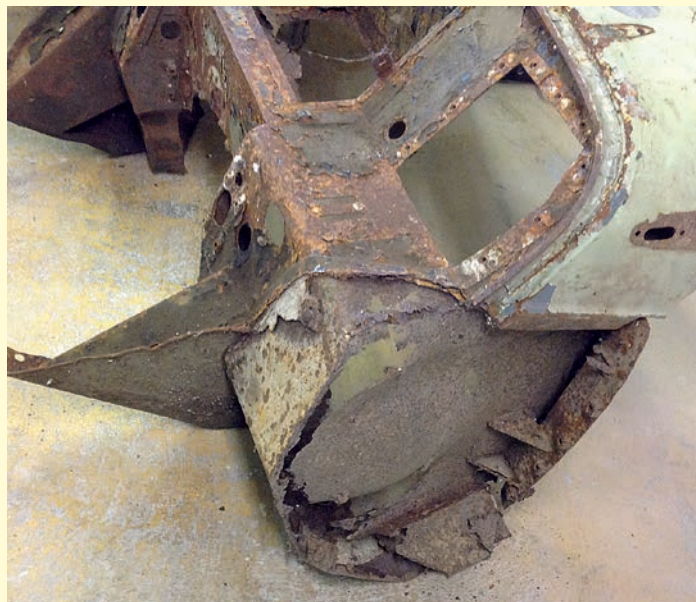
The car was nicknamed 'Lacy' as the metal was very thin in places – this shows what remained of the scuttle
