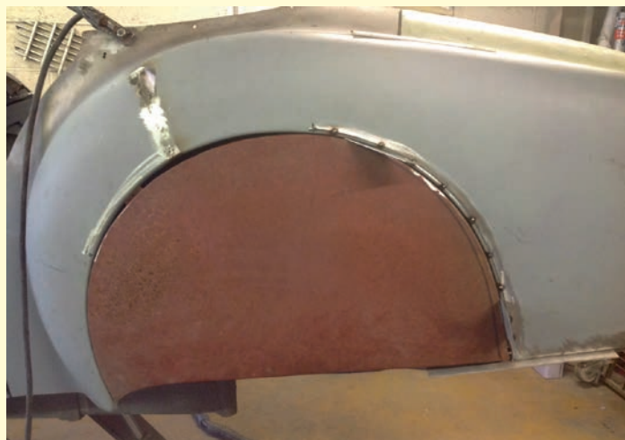
As many of the original parts as possible were retained; here the spats are being fitted to the front wings
